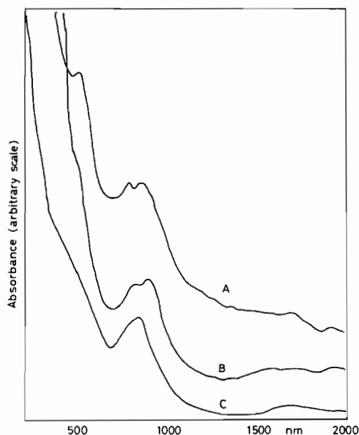
Fig. 4. Solid-state electronic spectra of the nickel complexes: A, \text{NiL}(\text{NO}_3)_2 ; B, \text{NiLBr}(\text{NO}_3) ; C, [\text{NiL}_2]\text{Y}_2 .
